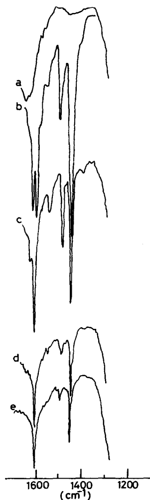
FIG. 11. Infrared spectra of pyridine adsorbed on Co(II)NaY-80. (a) Co(II)NaY-80 evacuated at 300°C for 1 hr; (b) pyridine was adsorbed at room temperature under 10 Torr and evacuated at room temperature for 15 min; (c) evacuated at 240°C for 30 min; (d) evacuated at 340°C for 1.25 hr; (e) evacuated at 360°C for 1 hr.
